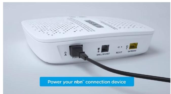
Plug the included grey telephone cable (B) into plug B (WALL SOCKET) on the back of the NCD. Plug the other end of the telephone cable (B) into your wall socket. You will now need to wait for the connection light and the DSL light on the top of the NCD to turn solid blue - this may take up to 15 minutes. **DO NOT UNPLUG THE DEVICE DURING THIS TIME.**
