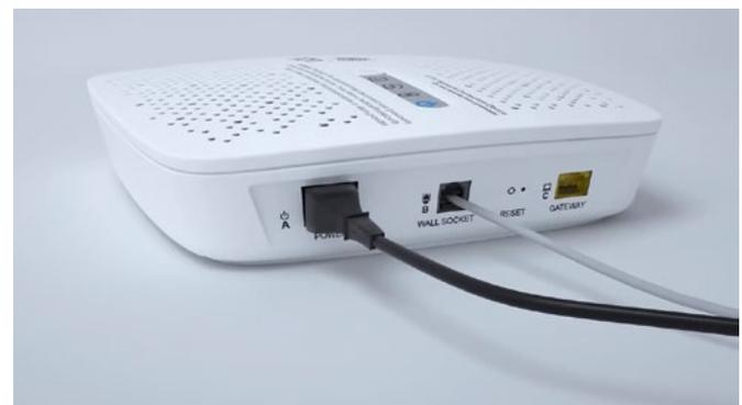
If the connection light and DSL light on the top of the NCD do not turn solid blue after 15 minutes and you have more than one socket in the home, please plug the NCD into other sockets in your home, and turn
